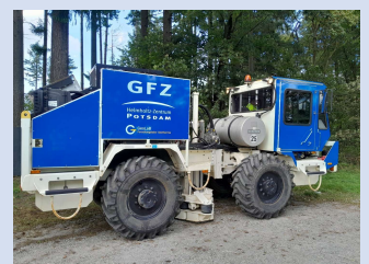
Figure 4. GFZ Vibroruck deployed during the recent pilot seismic campaign.
