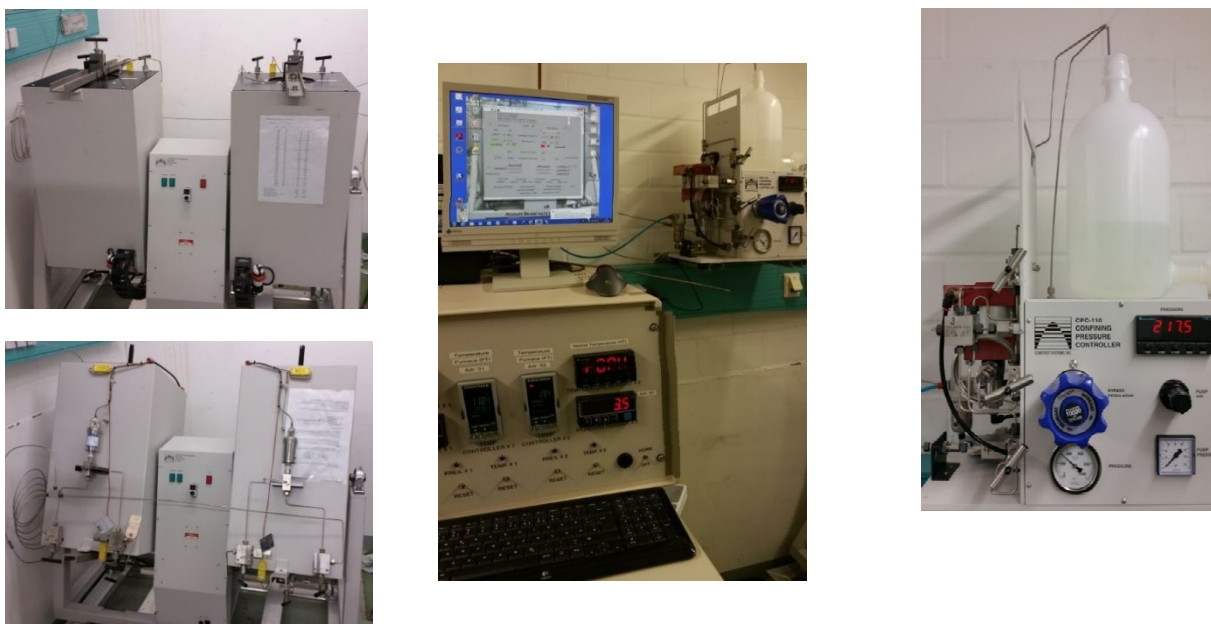
Fig 2: Rocking hydrothermal autoclaves at GFZ Potsdam; fully assembled autoclave (left), the monitoring unit (center), and the confining pressure controller (right)
