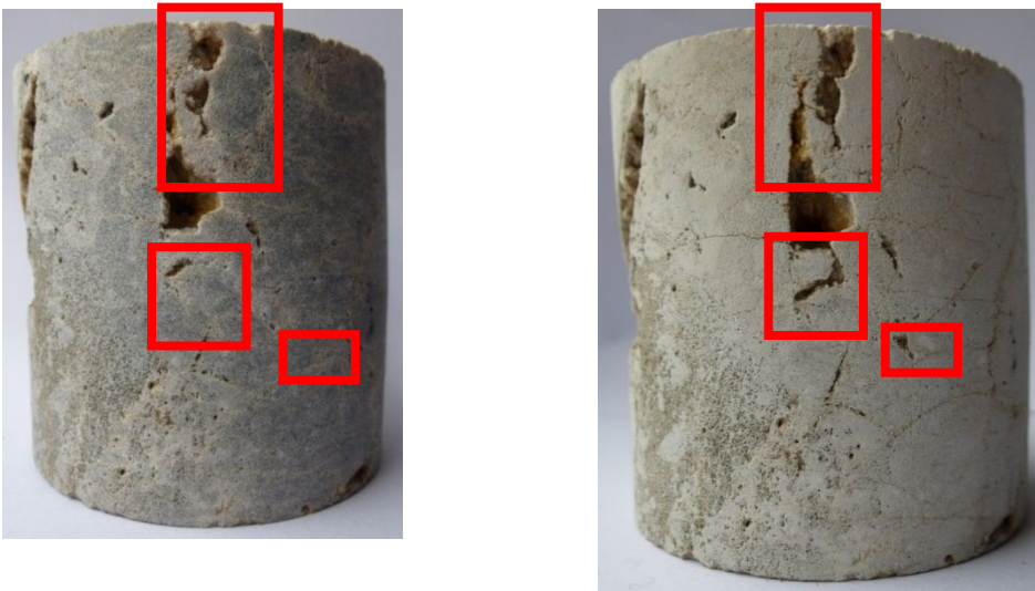
Fig. 8: Drill core sample before (left) and after (right) experiment. Clear signs of dissolution are visible on the edges of fractures and voids (red markings) [Anne Kaulisky].
