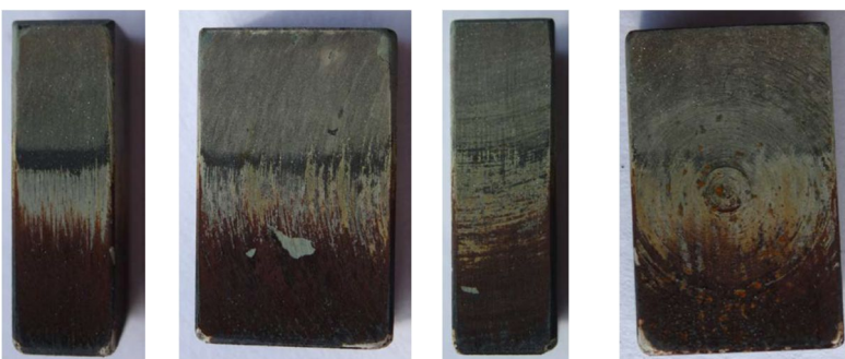
Fig 9: Casing material sample after experiment V012; red brown discoloration (probably iron oxide) is visible on the lower part [Anne Kaulisky].
