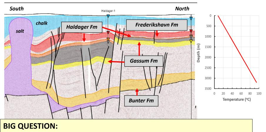
Which reservoir to develop for the production of geothermal energy?
