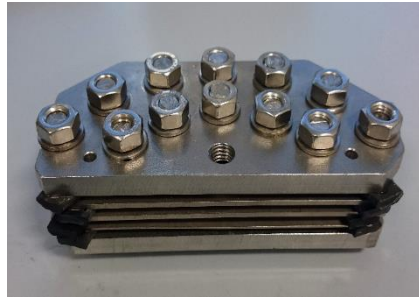
Pre-pressurized with 10 Nm tightening torque
