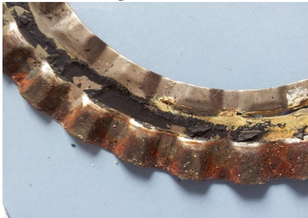
damaged sealing on Ti-plate
