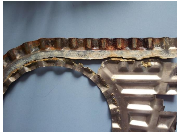
Severe corrosion (mispolarisation of Ti)
