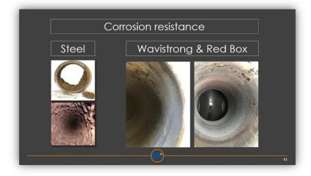
"Glass fibre reinforced epoxy pipes"
