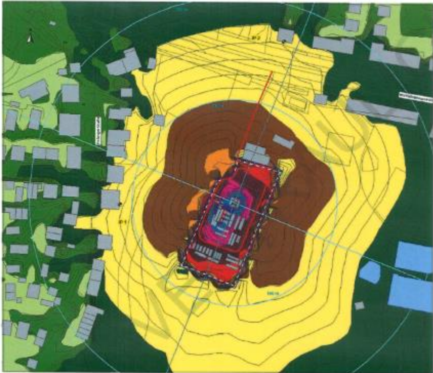
Bohranlage Terra Invader 350 t B002 Variante 4: Bohren, Immissionsraster
