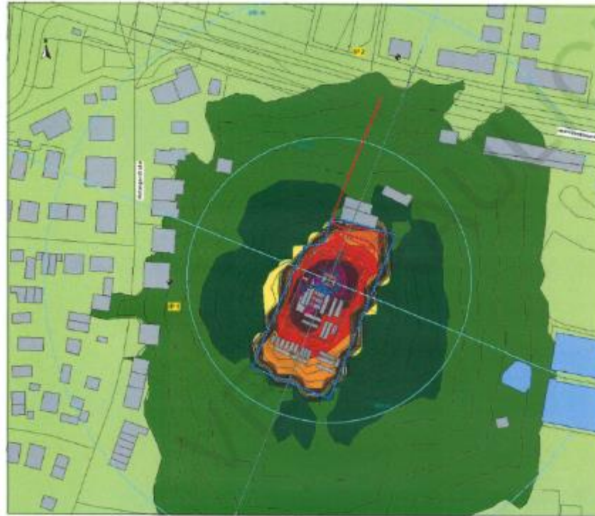
Bohranlage Terra Invader 350 t B002 Variante 7: Bohren, Immissionsraster
